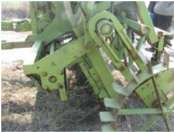
Prototype seeder for sowing wheat into heavy rice stubble featuring sickle bar cutters in front of every seeding tyne. The Punjab state has a strong agricultural engineering history.
