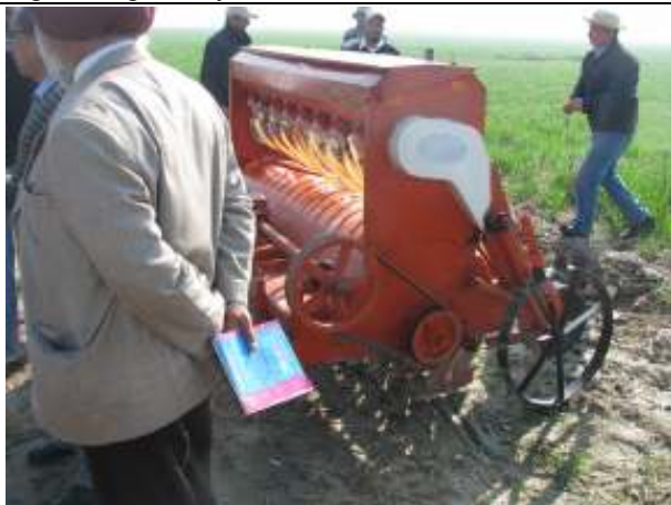
“Happy Seeder” developed for sowing into heavy rice stubbles, features a rotary slasher in front of each seeding tyne which clears a path for the tyne
